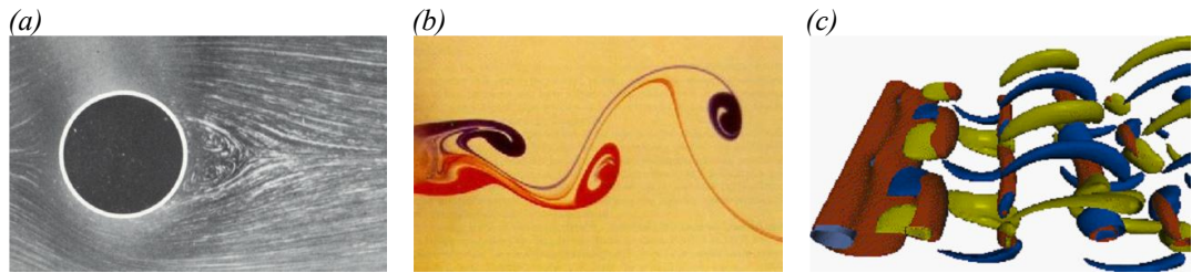
Instabilities developing in the wake of a circular cylinder. (a) The steady two-dimensional wake below Re = 46 (Van Dyke 1982), (b) the periodic two-dimensional Kármán vortex street above Re = 46 , and (c) the three-dimensional “Mode A” wake above Re \approx 190 (Thompson, Hourigan & Sheridan 1996).
